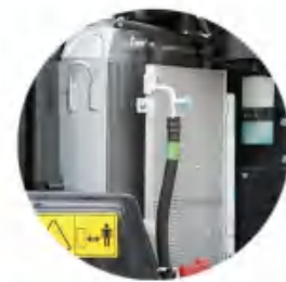
03 Water tank & radiator
