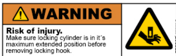
Figure 26. Warning decal on locking cylinder.
